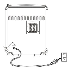
**Note:** This unit has a polarized AC plug with one wide blade and one narrow blade. This plug will only fit into a matching polarized AC outlet. This is a safety feature to reduce the possibility of electric shock.
